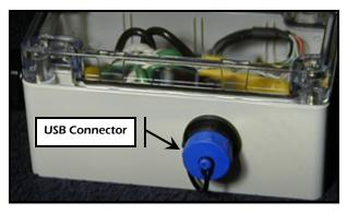
Sealed USB, panel mount connector. Provides water tight connection when used with optional MINI B to A USB cable.
